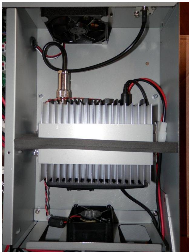
*DR1-X Repeater transmit side, with heat sink and push and pull cooling fans*
