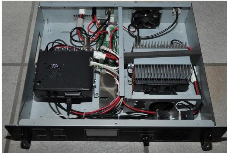
*DR1-X Repeater with top lid removed. Receiver is on the left, transmitter on the right.
